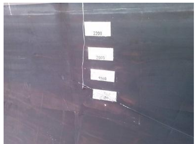
Draft marks (as-built)
